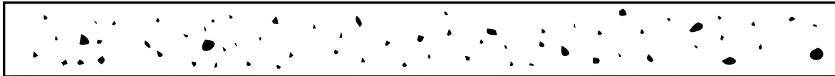
Figure IV-3-4 Charts for t Over 6.4 mm to 9.5 mm ( \frac{1}{4} in. to \frac{3}{8} in.), Inclusive
